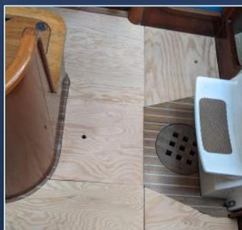
Once all the boards were cut and fit, I laid them out in our basement so I could ensure that the stripes were aligned along the fore and aft direction. Ensuring that the stripes were aligned at the transitions between the cabins was probably the most challenging aspect of the project. I sealed the bottom and edges of each board with West Epoxy to eliminate water penetration going forward. The vinyl was glued to the bare wood on the top to allow the penetration needed for good adhesion.
